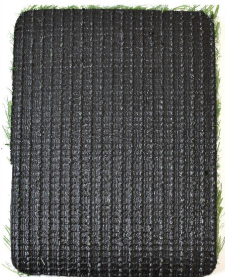
Adhesive backing: Secondary styrene butadiene latex
