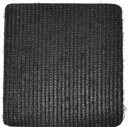
Adhesive backing: Secondary styrene butadiene latex
